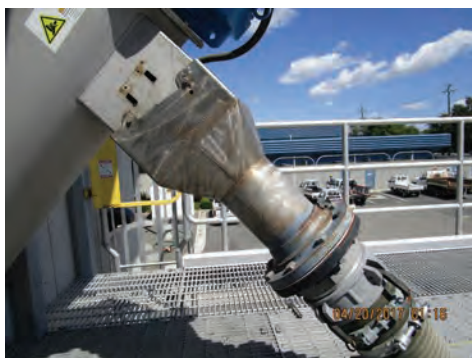
Figure 3: Top, smooth transition eliminates buildup points shown in bottom image
