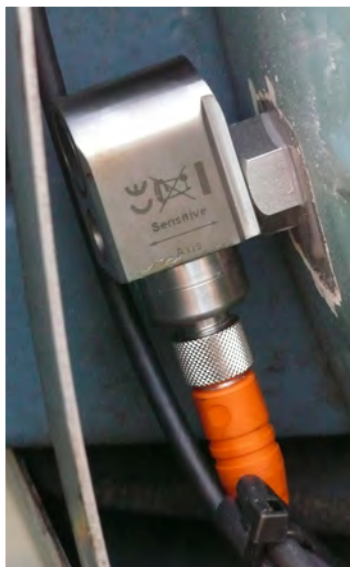
Figure 1: Accelerometers must be mounted securely on a clean and solid base and as close to the component being monitored as possible
