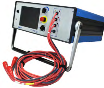
Figure 2: Surge and Hipot testing tests insulation between turns, coils, phase and to ground
